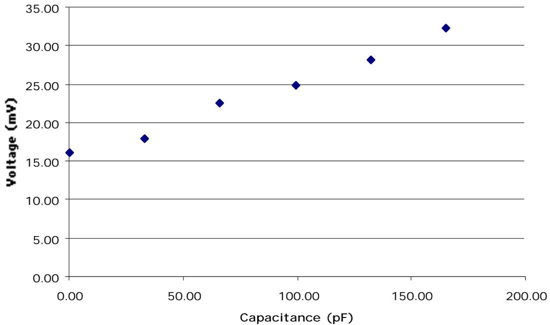
**Figure 3.** Voltage vs. Capacitance without the bypass capacitor.
