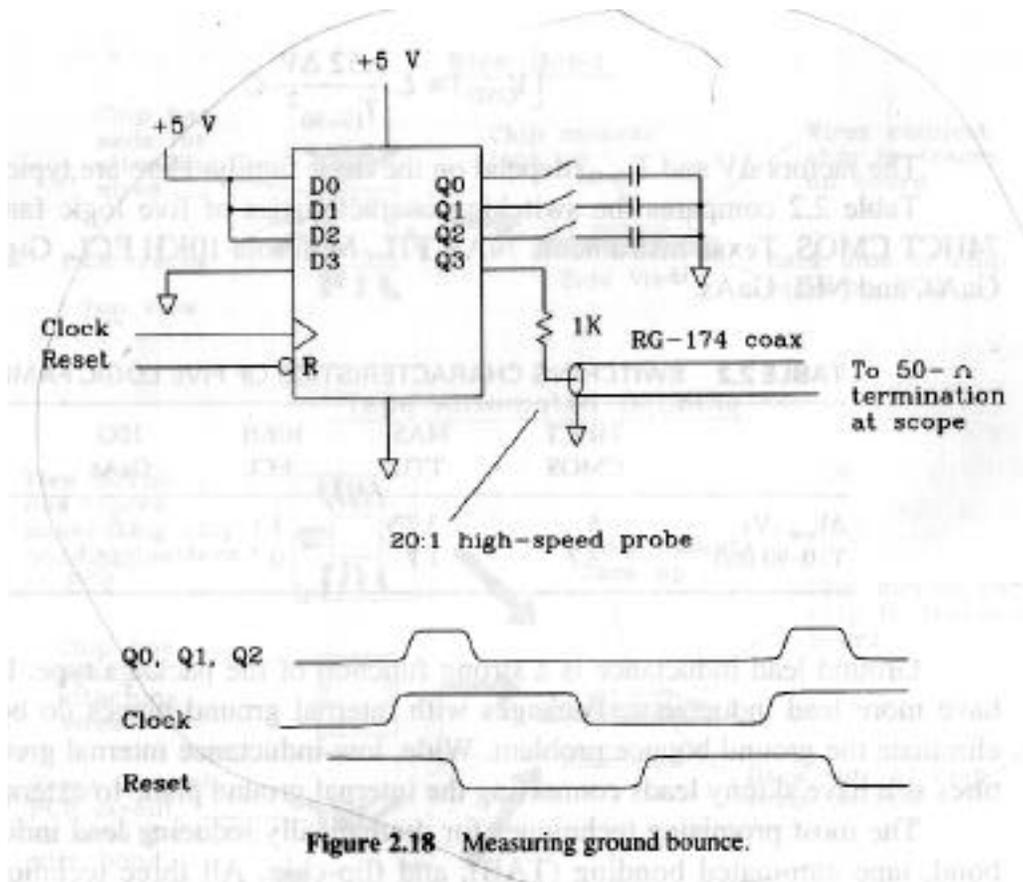
**Figure 1.** Ground bounce experiment design from the High Speed Digital Design text book.
